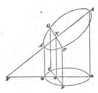
Take a chord PQ parallel to the plane of projection, then its projection pq = PQ.
